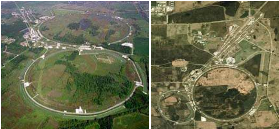
Figure 3.1: Aerial shot of the Fermilab site. Two rings of the accelerator system, the Tevatron and the Main Injector can be seen.
