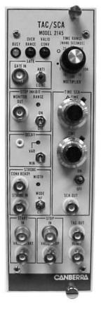
panel STOP INHIBIT adjustment allows rejection of STOP input signals in a range of 1% to 100% of each time range. This is useful for suppressing unwanted inputs in applications such as linear accelerators, and prevents false outputs. A MONITOR output is provided; when its output is true, STOP pulses are inhibited.
