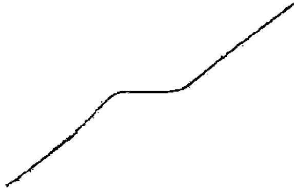
Figure 5-4 A typical Mr. SQUID ® V-I characteristic.
