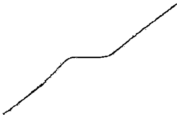
Figure 4-3 A typical Mr. SQUID ® V - I characteristic.
