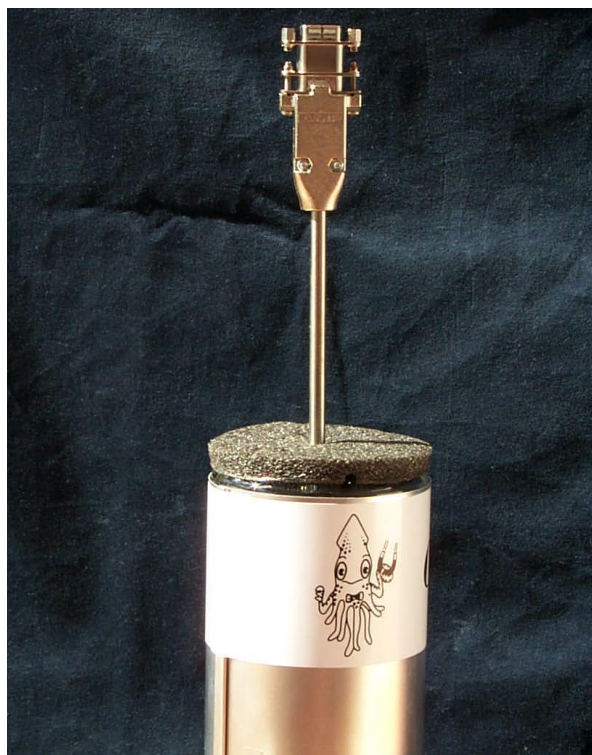
Figure 2-3 Mr. SQUID ® inserted into liquid nitrogen dewar.
