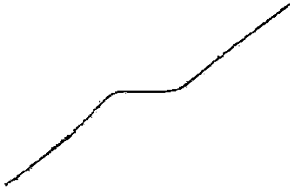
Figure 3-3 Typical Mr. SQUID ® V - I characteristic.
