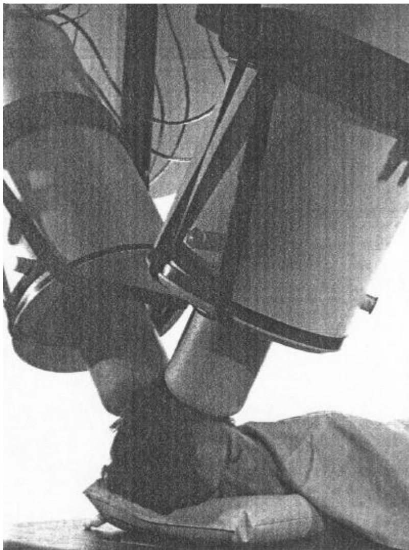
Biomagnetism. SQUIDS inside the two cryostats shown in this photograph detect magnetic fields emanating from the subject's brain. Each cryostat contains seven second-order gradiometers to detect the signal, and three magnetometers and one first-order gradiometer for electronic cancellation of background noise. The sensors are immersed in liquid helium, which is contained by the superinsulated fiberglass cryostats. (Photograph by Hank Morgan, courtesy of New York University Medical Center and Biomagnetic Technologies Inc.) Figure 1
