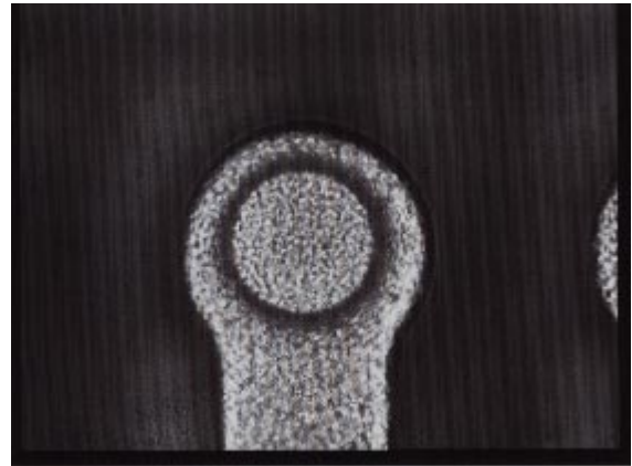
Figure 8: Top view of a via in the Photo-BCB with a diameter of 25 \mu m mask dimension (video print)
